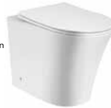
D218 Floor Standing Toilet Flushing system: Washdown Size: 555x365x410mm Vitreous china P trap: 1 80mm Fixing to wall with back
